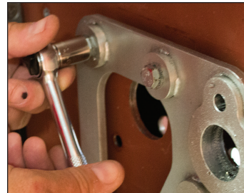
10 - Remove Fixture with 1/2" socket wrench
