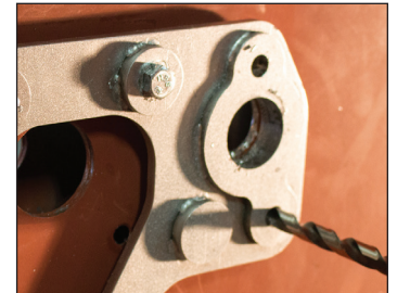
9 - Base Plate Side Drill Wire Entry Hole
