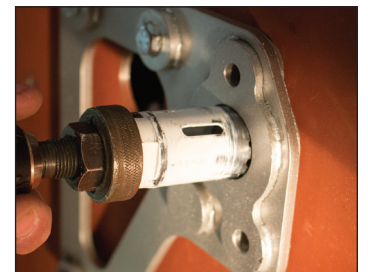
5 - Drilling Back Template Rim Cylinder Hole
